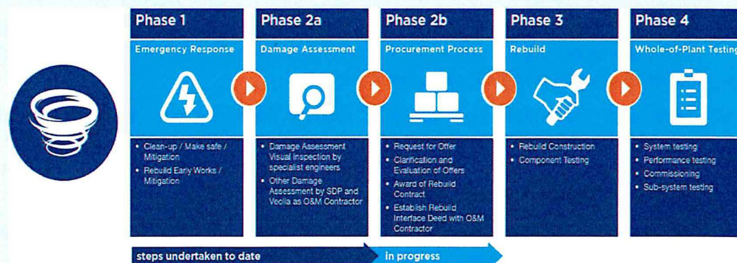
Figure 3: Responding to damage caused by the December 2015 Sydney Tornado
