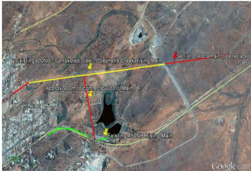
Figure 1.4: Possible temporary cross connection between the Stephens Creek to Broken Hill pipeline
