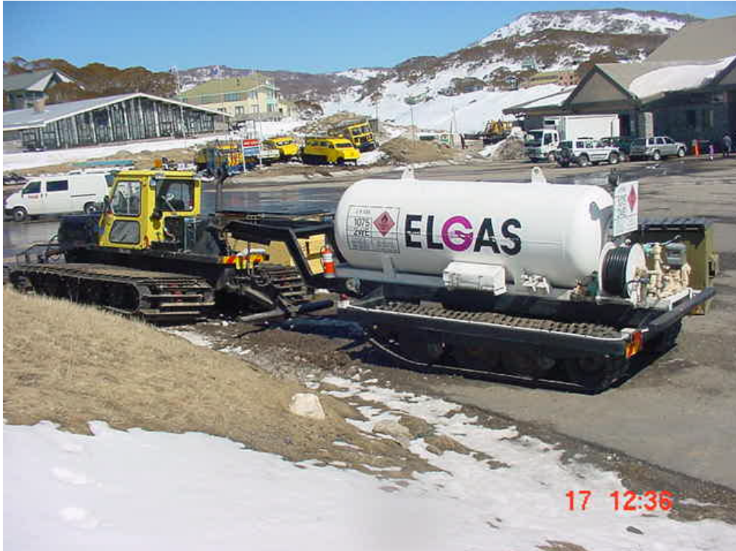
PHOTOGRAPH No.3. Over snow bulk LPG tank – In front of Ski tube station
