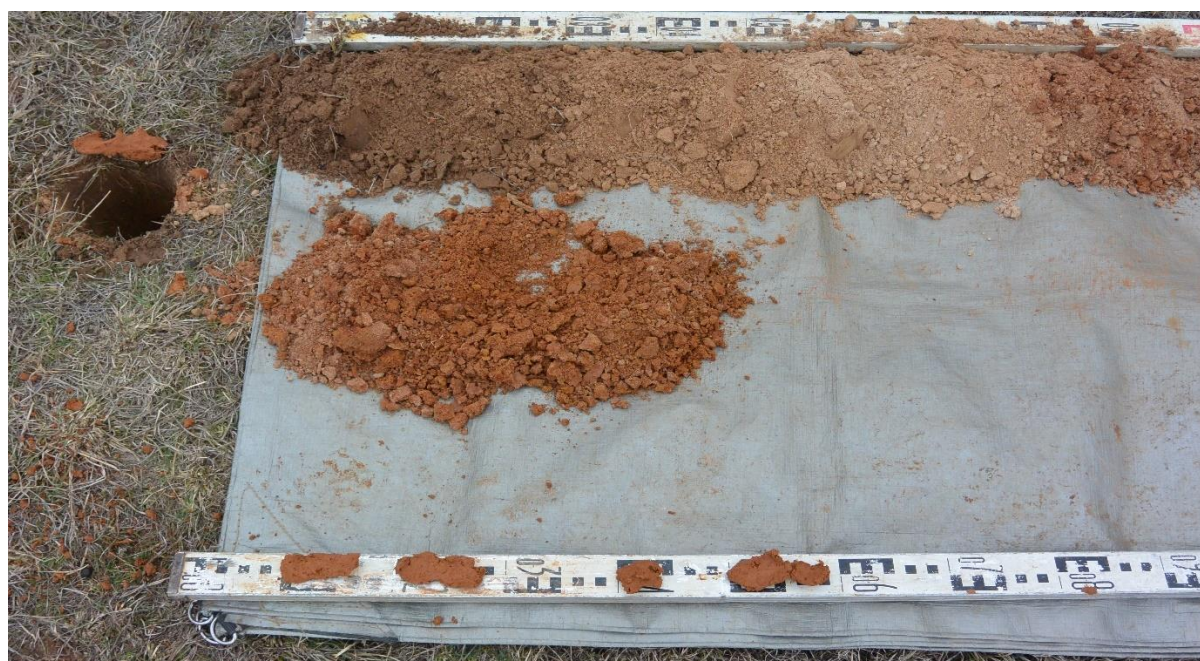
Figure 12: Soil Texture Field Analysis – Ribbon length 70mm – Light Clay
