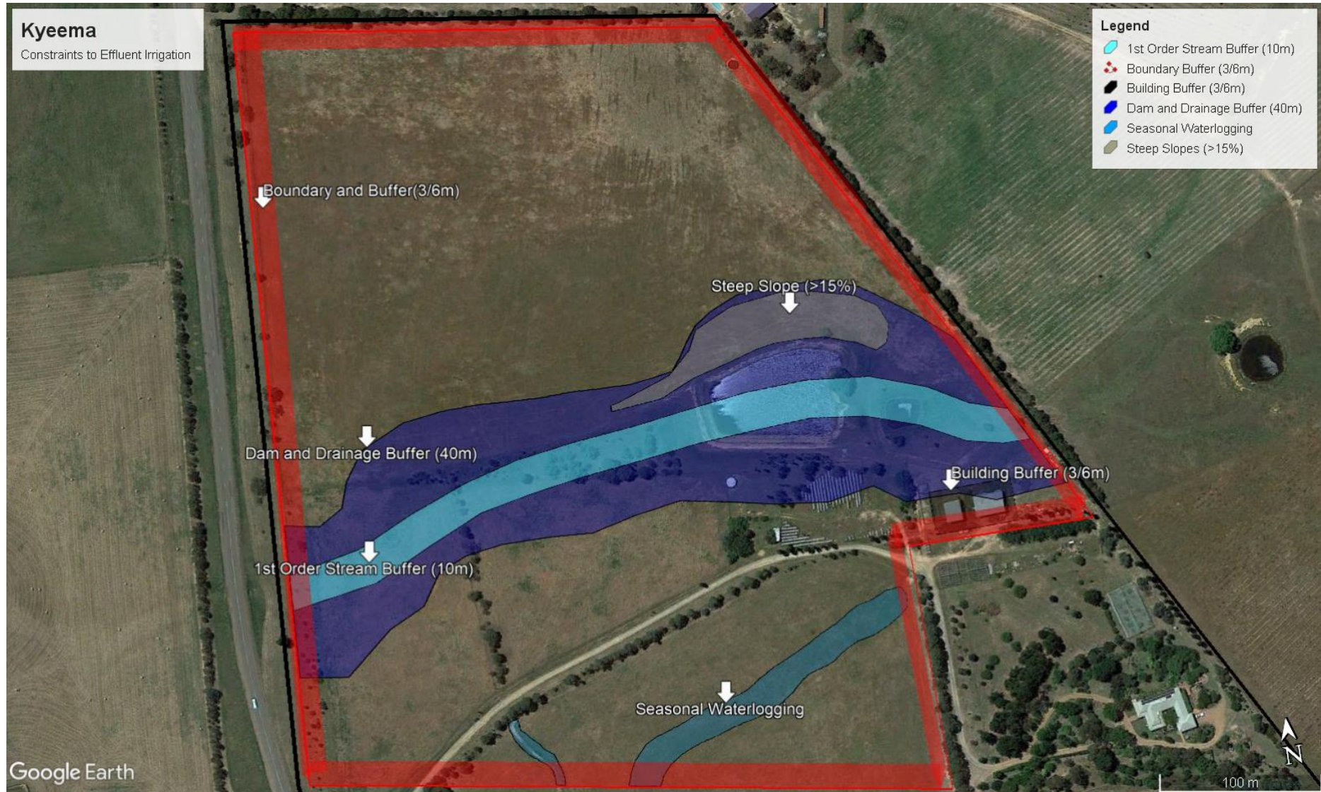
Figure 7b: Effluent irrigation area constraints – unconstrained areas are suited to effluent irrigation practices
