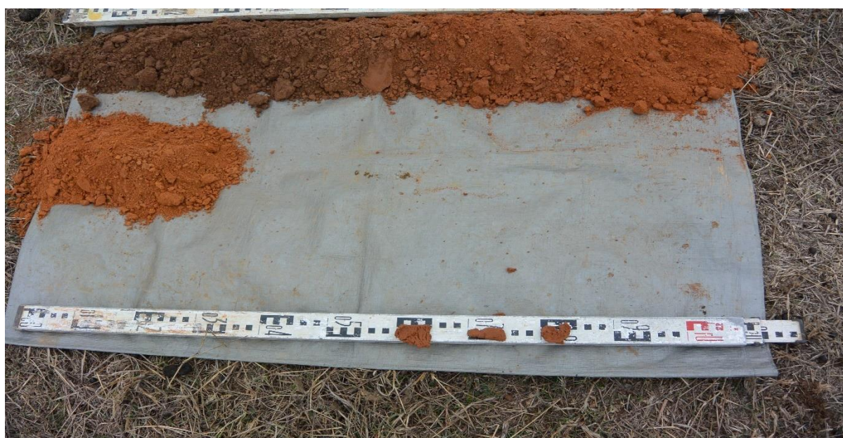
Figure 10: Soil Texture Field Analysis – Ribbon length 50mm – Sandy Clay Loam
