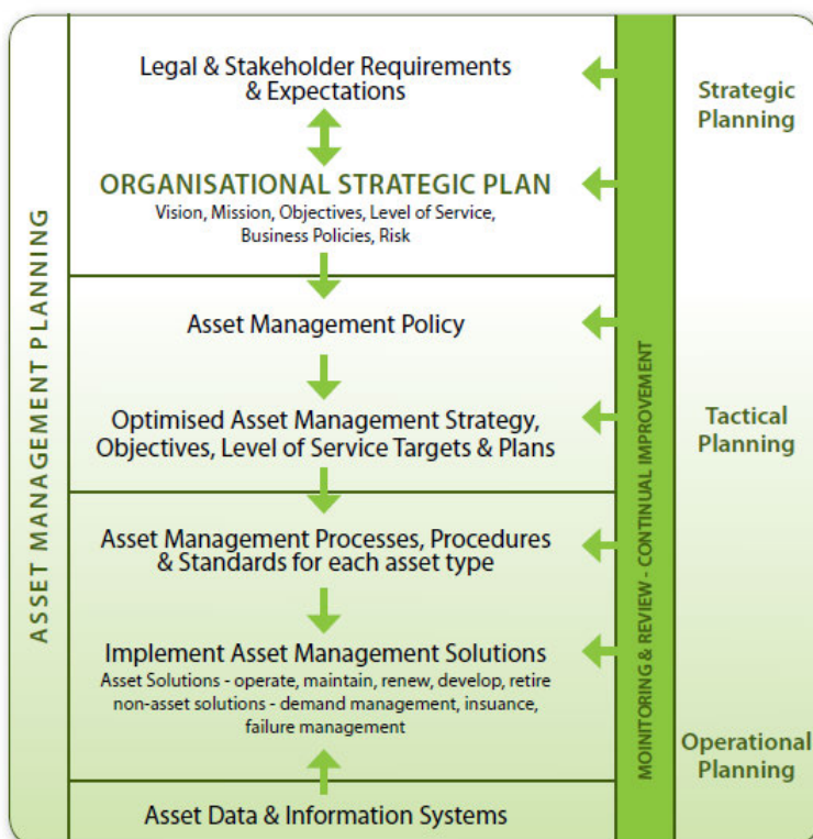
Figure 1 Goulburn Mulwaree Asset Management Planning Framework
