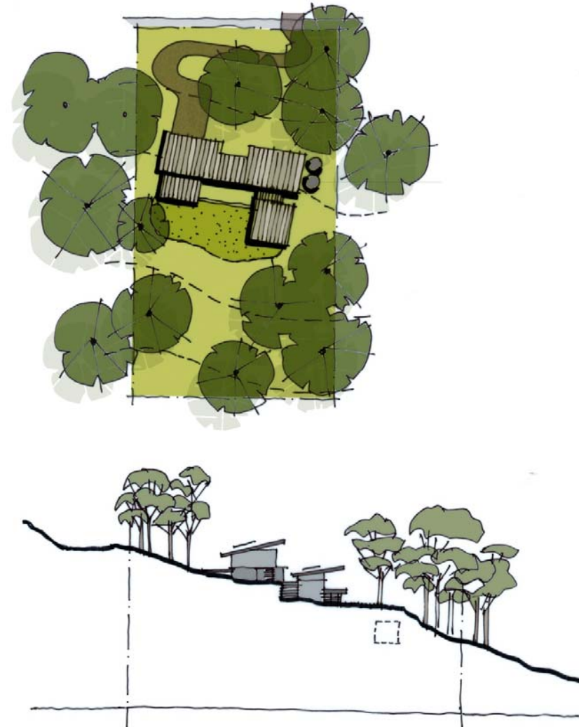
Figure 4.16 Layout of Rural Residential Dwelling responding to topography and slope Source: HASSELL 2009
